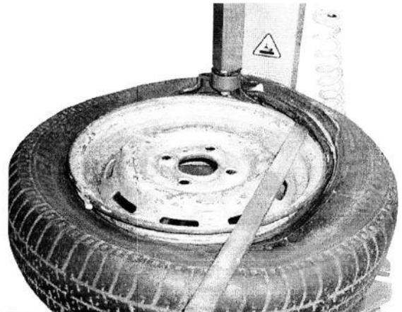
**Fig. 11 Removing tyre**
