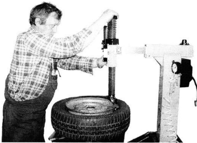
**Fig. 8 Setting working head**
