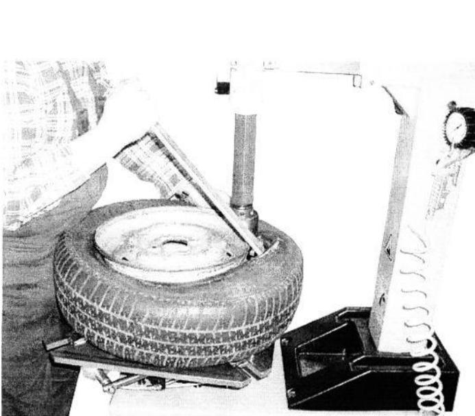
**Fig. 10 pulling tyre edge onto shoe**
